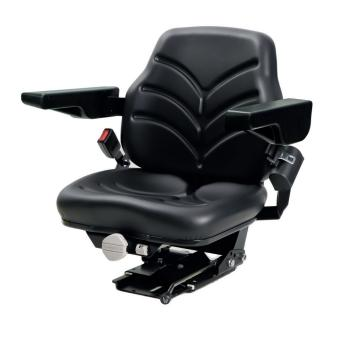
Mechanical suspension Weight adjustment Manual up to 130kgs. Suspension stroke 80mm Height adjustment 60mm Slide travel 150mm Fold-up armrests Backrest adjustment N/A Vinyl trim (Vacuum type) Cloth trim (Vacuum type) 2-point seat belt Document pouch Operator presence switch EU 1322/2014 Annex XIV - Class I, II - ECE R16.08 - ISO 3795
