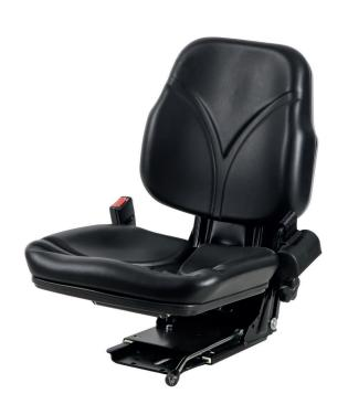
Mechanical suspension Weight adjustment Manual up to 130kgs. Suspension stroke 80mm Height adjustment 60mm Slide travel 150mm Fold-up armrests Backrest adjustment N/A Vinyl trim (Vacuum type) Cloth trim (Vacuum type) 2-point seat belt Document pouch Operator presence switch Testing EU 1322/2014 Annex XIV - Class I, II - ECE R16.08 - ISO 3795
